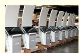
Generally, the ideal quantity for production after prototype should be 20 units or more. At this level with sheet metal, the setup fees for all of the CNC equipment required to build the kiosks, begin to have an economy of scale.
