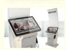
In order to create our computer renderings, we first start by creating a wire frame using SolidWorks. When possible, we use manufacturer provided 3D CAD data of all PCs, monitors and other peripherals used in the kiosk.
